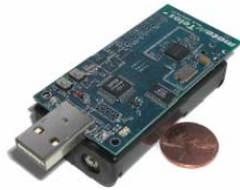
Figure 2: Telos ultra low power mote with IEEE. 802.15.4 wireless transceiver.
