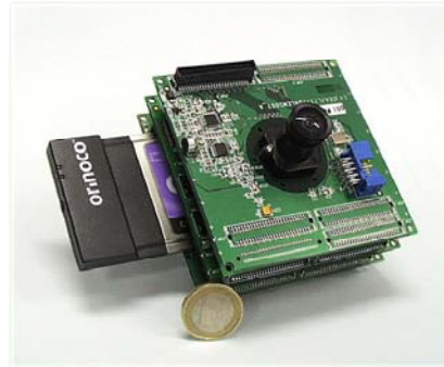
Fig 3 Prototype design of the wireless sensor node
